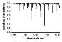
**Methane Absorption Spectrum** (CQ09075-CH4)
