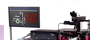
**MPM200-4** Four-Channel Multiphoton System shown on a PHYS24M Physiology Stage with MPM-BCU Beam Conditioner and COMP6300 Dispersion Pre-Compensation Units, all placed on a 5' x 6' SDA150180 ScienceDesk<sup>TM</sup>.
