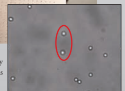
Simultaneously Trapped 1 \mu m Beads
