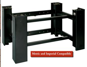
This family of passive isolation systems incorporates four independent air mounts for general applications requiring isolation from low frequency vibrations. Each leg is manually controlled to achieve a level surface and does not require a constant source of air to maintain the setting. A manual foot pump such as our PTA126 (see page 72) is recommended for pressurizing passive vibration isolation systems.
