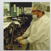
Pigtailed Laser Diode Alignment
