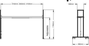
Freestanding Shelf works with all of our breadboard units and does not interfere with vibration isolation. Available in three sizes.
