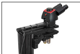
Figure 8.3 The mounted LED and epi-illuminator module attached to the Cerna microscope.
