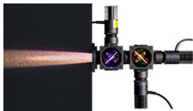
Figure 6.7 Beam Profile of Source with 3 Mounted LEDs
