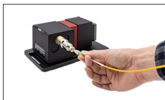
Click to Enlarge Step 1: Connect the included FC/APC fiber to the spectrometer.
