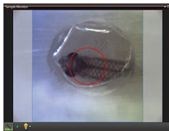
Click to Enlarge A predefined circle scan pattern can be loaded and scanned in the software. The size can be changed with the Zoom feature.
