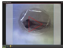
Click to Enlarge A predefined triangle scan pattern can be loaded and scanned in the software. The size can be changed with the Zoom feature.
