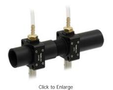
This air circulation unit purifies air in three separate stages. First, air is passed through the Desiccant Filter designed to trap airborne water molecules. Next, air is passed through the 15  $\mu$ m Particulate Filter which removes particulates with better than 95% efficiency. The final filter is the 13X Molecular Sieve, which traps volatile organic compounds. Replacement filters can also be purchased separately below.
