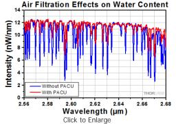
The graph above shows the water absorption spectrum of a boradband halogen source coupled to an OSA205C Optical Spectrum Analyzer through free space. The blue trace shows the spectrum without the air purification while the red shows the spectrum with air purification used to purge the OSA205C cavity. The use of the PACU Pure Air Circulator Unit reduces the water absorption inside the OSA.
