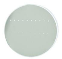
The photograph above is a protected aluminumcoated mirror after LIDT testing. In this particular test, it handled  $0.43 \text{ J/cm}^2$  (1064 nm, 10 ns pulse, 10 Hz,  $\emptyset$ 1.000 mm) before damage.
