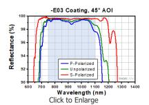
Excel Spreadsheet with Raw Data for -E03 Coating, 6° and 45° AOI
