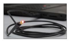
A LED630L being powered by the USB port in a laptop.
