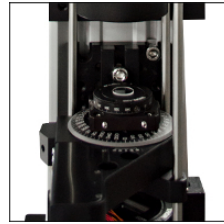
Figure 3: The test setup for checking the retardance and alignment uniformity of our vortex retarders.
