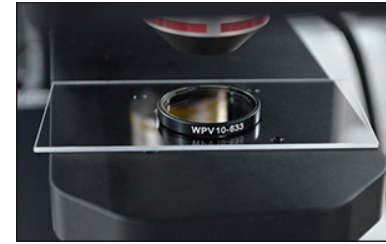
Figure 5: A close up of a vortex retarder in one of the test setups.
