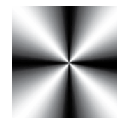
The intensity profile created by an m = 2 retarder when viewed between crossed polarizers.
