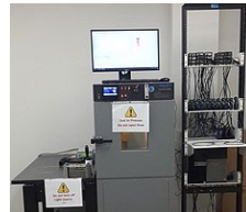
Click To Enlarge Damp Heat Testing Setup
