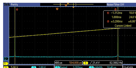
Figure 1: An FSR Plot, Using a 1550 nm DFB Laser (PRO8000 Series). Using the SA200-12B
