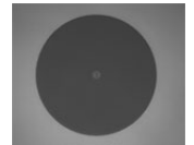
Undamaged Fiber End
