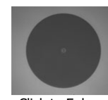
Click to Enlarge Undamaged Fiber End
