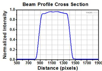
Top-hat beam profile measured using lenses to expand the beam.
