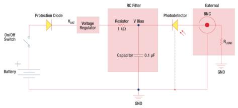
Figure 2: Reverse-Biased Circuit (DET Series Detectors)
