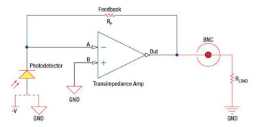
Figure 3: Amplified Detector Circuit
