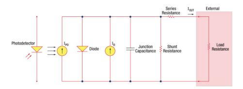
Figure 1: Photodiode Model
