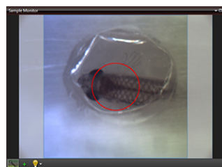
Click to Enlarge A predefined circle scan pattern can be loaded and scanned in the software. The size can be changed with the Zoom feature.
