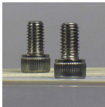
Figure 5: The same two screws photographed with our MVL7000 conventional zoom lens. In this image, the perspective error due to the separation of the screws would lead to incorrect height measurements.
