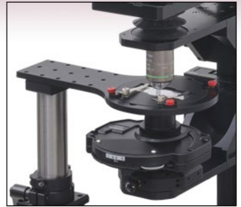
MP200-RCH2 Adjustable Stand Shown Holding a Microscope Slide Between an Objective and Condenser
