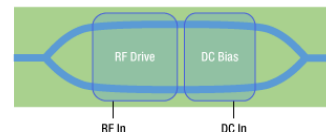
Click to Enlarge This operational diagram of an intensity modulator shows the waveguide (blue lines) splitting into two
