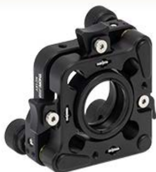
KC1XY SM1 (1.035"-40) Tap in Front Slip Plate
