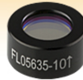
FL05635-10 Ø1/2" Filter CWL = 635 nm, FWHM = 10 nm
