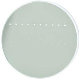
The photograph above is a protected aluminum-coated mirror after LIDT testing. In this particular test, it handled 0.43 J/cm<sup>2</sup> (1064 nm, 10 ns pulse, 10 Hz, Ø1.000 mm) before damage.
