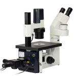
Click to Enlarge Multi-LED Source Coupled to Microscope Illumination Port
