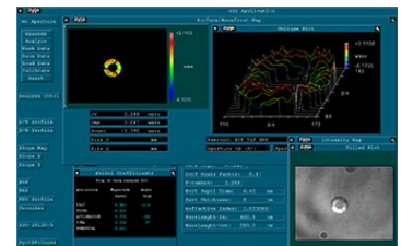
Click to Enlarge LMM40X-UVV Interferogram with Measured Seidel Coefficients
