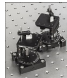
Figure 3: Anamorphic Prism Pair System
