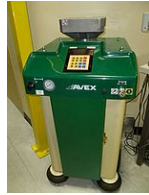
To Enlarge SM-105 Mechanical Shock Test Machine
