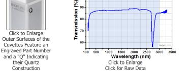
Transmission of UV Fused Quartz Cuvette
