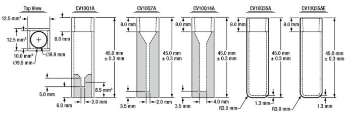
a. ±0.2 mm for Standard Cuvettes; +0.0/-0.2 mm for Cuvettes with Enhanced Chemical Resistance
