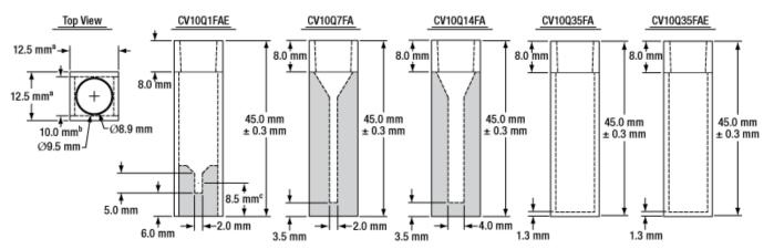
a.  $\pm 0.2$  mm for Standard Cuvettes;  $\pm 0.0/-0.2$  mm for Cuvettes with Enhanced Chemical Resistance b.  $\pm 0.08$  mm for Standard Cuvettes;  $\pm 0.05$  mm for Cuvettes with Enhanced Chemical Resistance
