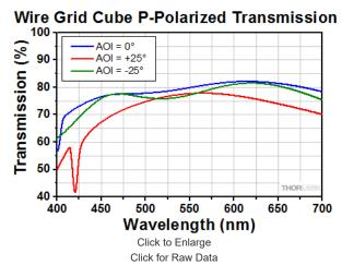
The graph above shows the measured transmission through the wire grid polarizing cube for p-polarized light for light incident upon one of the entrance faces. The plotted data is given for AOIs of 0° and ±25°.
