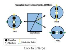
then the light will be deviated by the prism such that it emerges from port 2 with the light aligned to the slow axis. Note that the slow axes of the fibers on port 1 and port 2 are orthogonal to each other to match the polarization emitted by the calcite prism. If the polarization incident on port 3 is at an angle with respect to the axes, the output at ports 1 and 2 will vary depending on the angle of the incident polarization state.
