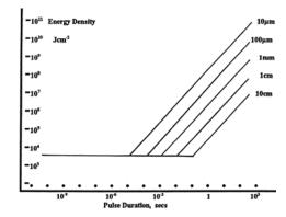
LIDT in energy density vs. pulse length and spot size. For short pulses,
