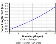
LA 7542-G Ø1" Lens, f=25.4 mm, 7-12 μm AR Coating
