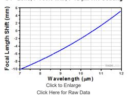
LA 7028-G Ø1" Lens, f=150.0 mm, 7-12 μm AR Coating
