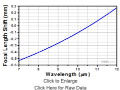
$$LA\,76\,56\text{-}G$$  Ø1" Lens, f=50.1 m m , 7-12  $\mu m$  AR Coating
