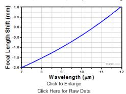
LA7270-G Ø1" Lens, f=500.0 mm, 7-12 μm AR Coating
