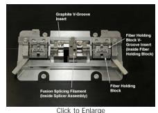
The locations of the components that can be purchased separately are labeled in the schematic above and are available for purchase below. An FTV7 Tungsten filament and two VHG125 Graphite V-Grooves come pre-installed with each FSX2000PM). For more details, please see the list to the left and the *Decisions* tab.
