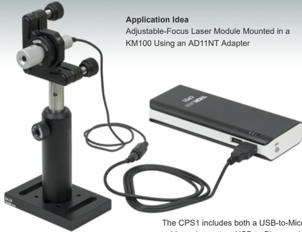
The CPS1 includes both a USB-to-Micro-USB cable and a custom USB-to-Phono cable.
