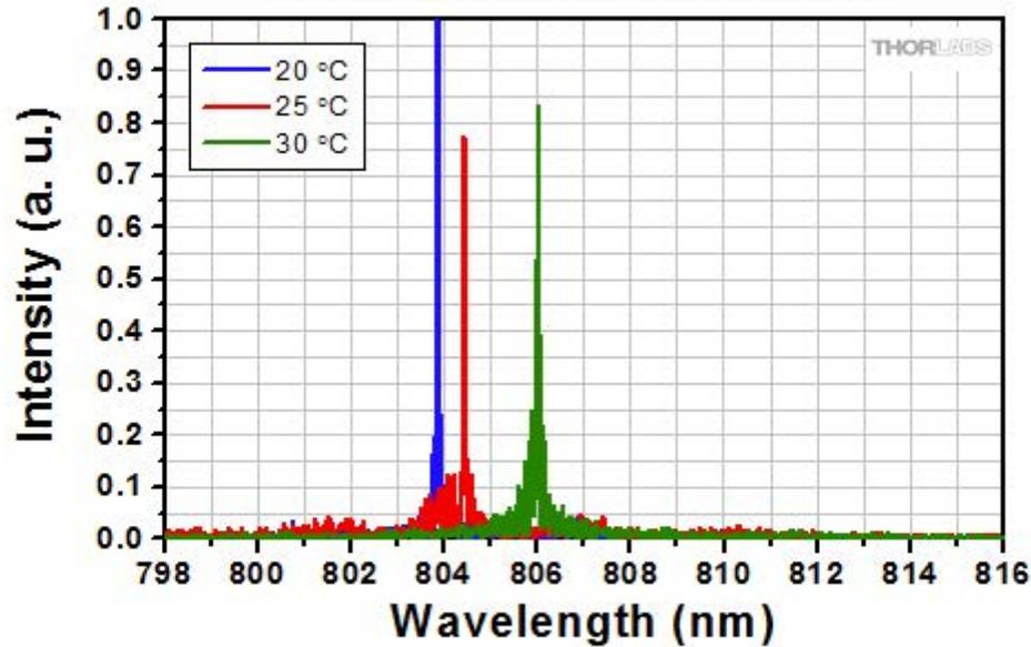
Spectrum of the CPS808A Diode Module taken at 20 °C, 25 °C, and 30 °C. The measurement was taken using Thorlabs [OSA201 Spectrum Analyzer](#), which has a resolution of 7.5 GHz ( $0.25 \text{ cm}^{-1}$ ). This data is typical and will vary for each module.
