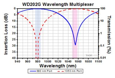
This plot shows an example of the spectral performance of a 980 nm / 1053 nm WDM. The lines represent the spectral response of each channel, while the blue and red shaded regions denote the bandwidth around each channel. This data is typical; performance of each coupler may vary within the coupler specifications. Data was obtained without connectors.
