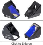
Click to Enlarge Thorlabs' filter cubes (top) retain the dichroic beamsplitter using a spring plate that applies force evenly, putting less stress on the optic compared to OEM cubes (bottom). The spring plate is also premounted on the cube, simplifying the assembly process.
