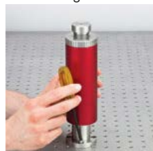
Click to Enlarge Step 2: Raise the red cover and attach the post base to the table.
