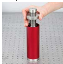
Click to Enlarge Step 3: Lower the red cover, ensuring the dowel pins in the base are aligned with the holes in the cover. Adjust the post to the desired height, and then lower the locking ring to lock the height.
