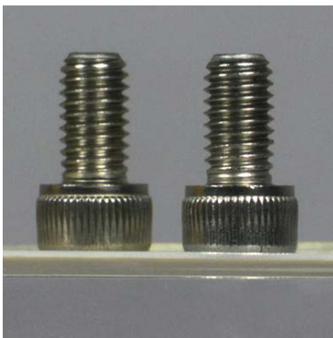
Figure 4: An image of two identical 8-32 cap screws imaged with our MVTC23013 0.128X Telecentric Lens. Although the screws appear to be the same size and in the same object plane, they are actually separated by a distance of approximately 45 mm along the optical axis.
