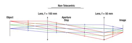
Figure 3: A ray trace through an idealized conventional camera lens system. Note that the chief rays (the center ray of each color) is not parallel to the optic axis in both image and object space, which means that the magnification will vary with object distance.
