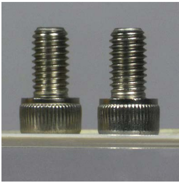
Figure 4: An image of two identical 8-32 cap screws imaged with our previous generation MVTC23013 0.128X Telecentric Lens. Although the screws appear to be the same size and in the same object plane, they are actually separated by a distance of approximately 45 mm along the optical axis.
