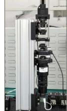
Click to Enlarge Custom Liquid Crystal Cell Test Setup
