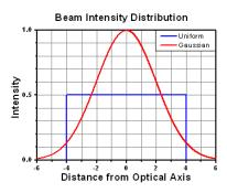
The calculation above assumes a uniform beam intensity profile. You must now consider hotspots in the beam or other non-uniform intensity profiles and roughly calculate a maximum
