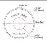
To operate as a light intensity modulator or shutter, again find the minimum transmitted intensity as prescribed above. Once the minimum is found, rotate the retarder by ±45°. This will maximize the transmitted intensity through the crossed polarizers for most LC retarders (e.g., zero-order quarter- or half-wave plates). However, this rule of thumb does not rigidly hold for multi-wave phase retarders using broadband sources due to the wavelength dependency of the retardation.
