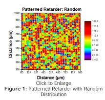
resolution of <1°. Figures 1 - 3 show examples of our patterned retarders. The figures represent measured results of the patterned retarder captured on an imaging polarimeter and demonstrate that the fast axis orientation of any one individual microretarder can be controlled deterministically and separately from its neighbors.
