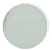
The photograph above is a protected aluminum-coated mirror after LIDT testing. In this particular test, it handled  $0.43~\mathrm{J/cm^2}$  (1064 nm, 10 ns pulse, 10 Hz, Ø1.000 mm) before damage.
