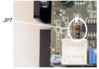
Servo driver cards manufactured after October 2009 have a jumper which is used to set the Volts per Degree scaling factor. The cards are shipped with the scaling set to 1.0 V/°, where the max scan angle is 10°, and is compatible with driver cards manufactured before October 2009.
