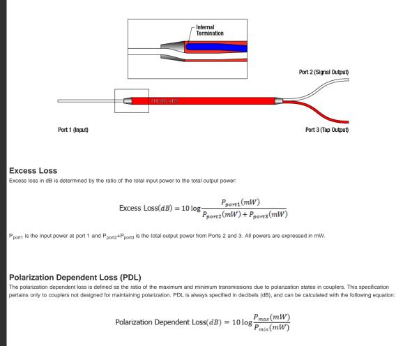
where  $P_{max}$  is the maximum power able to be transmitted through the coupler when scanning across all possible polarization states.  $P_{min}$  is the minimum transmission across those same states.
