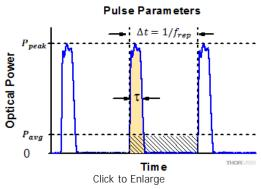
**Figure 1:** Parameters used to describe pulsed laser emission are indicated in the plot (above) and described in the table (below). **Pulse energy (E)** is the shaded area under the pulse curve. Pulse energy is, equivalently, the area of the diagonally hashed region.
