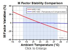
The above plot shows sample data comparing the M factor stability of our temperature-compensated avalanche photodetectors to our standard packages. The blue shaded region indicates the temperature range over which the M factor stability is guaranteed to within ±3%.
