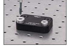
Click to Enlarge Once the TTT001(M) guide is properly aligned over the hole, use the TW25 Hand Tap Wrench with a 1/4"-20 tap (Item # 71598) or an M6 tap (Item # 71498) to restore the threads.
