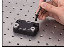
Click to Enlarge To repair a hole with the TTT001(M) guide, first secure it to the optical table using the included countersunk screws. These screws are designed to center the steel bushing over the damaged hole.
