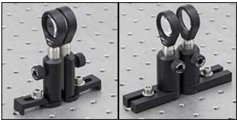
Click to Enlarge Close-Approach Post Holders can Mount Ø1/2" Posts in Contact, while Posts Mounted in Standard Post Holders are Separated by a Minimum of 0.48" (12.2 mm)
