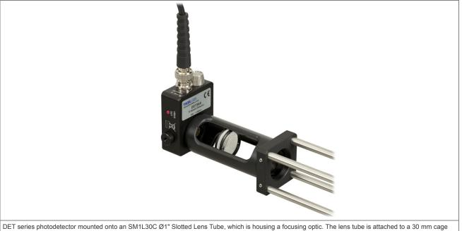
be I series photodetector mounted onto an SM1L30C Ø1" Slotted Lens Tube, which is housing a focusing optic. The lens tube is attached to a 30 mm cage system via a CP02 SM1-Threaded 30 mm Cage Plate. This arrangement allows easy access for optic adjustment and signal alignment.
