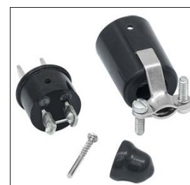
Step 4 Click to Enlarge Third, remove the protective cap to expose the short wire, which can be unsoldered.
